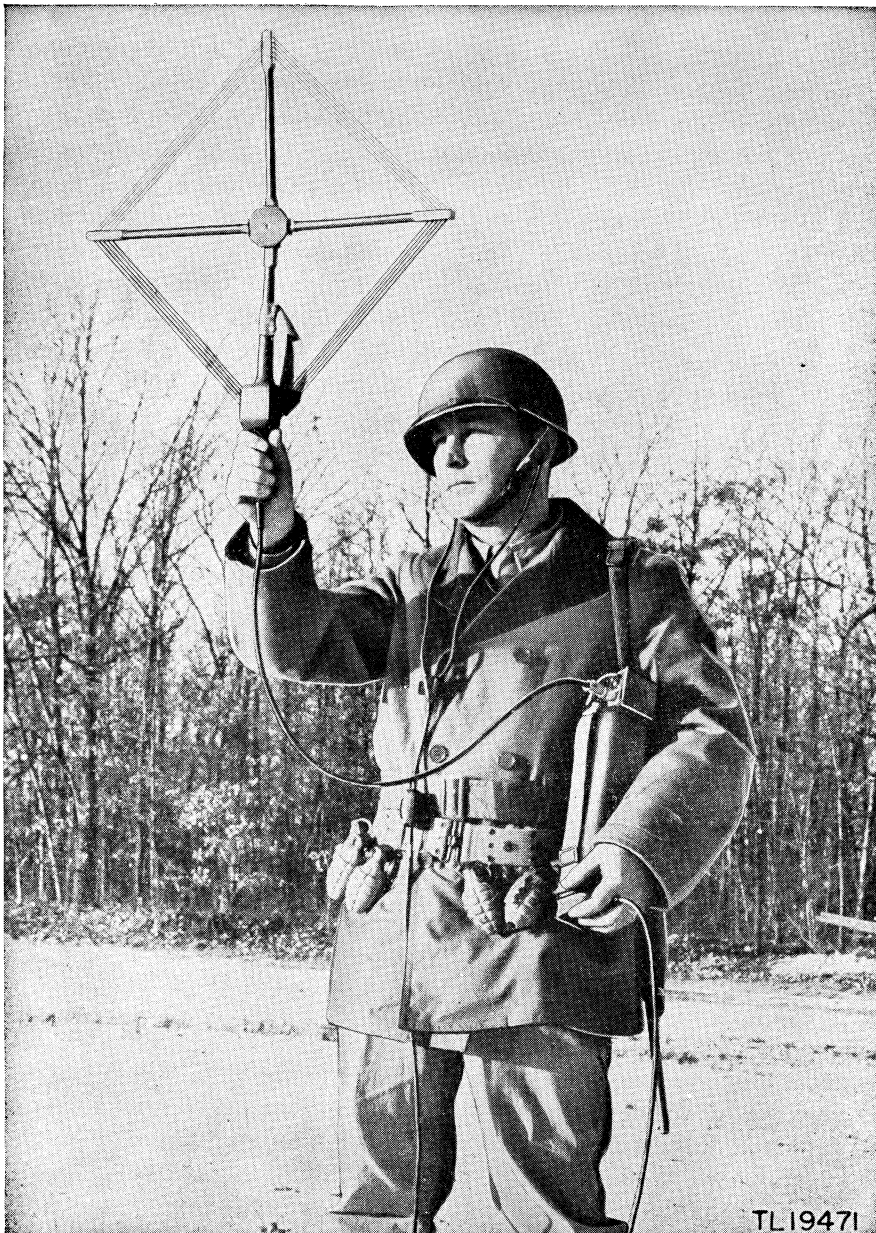
Figure 36. Homing Modification Kit MC-619 attached to Radio Receiver and Transmitter BC-611-(*).
